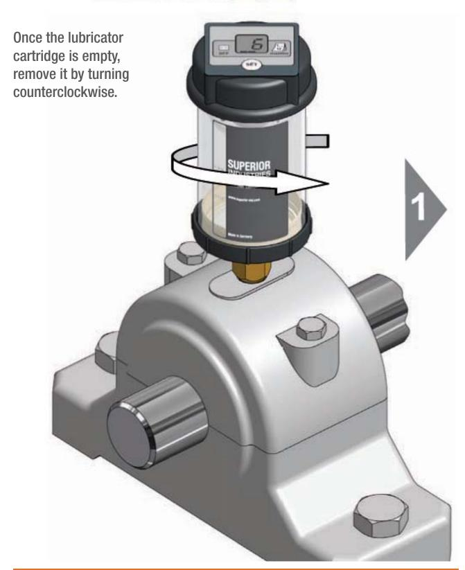
Remove the cap by turning it counterclockwise. Install the re-useable cap onto the new lubricator cartridge by pushing down and turning clockwise.
