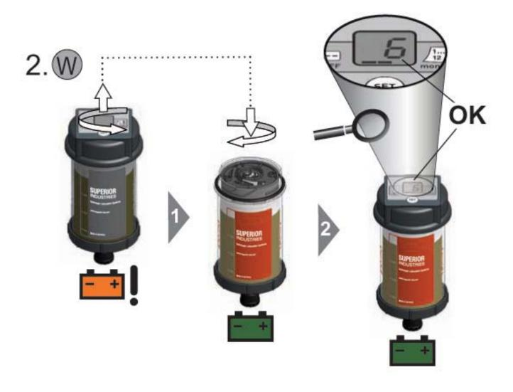
12 different dispensing rates are available (1-12). 1 means that the contents of the cartridge will empty over a one month period, (approximately 4.2cc/day for one 130cc cartridge OR 8.4cc/day for two cartridges on one grease zerk.) 2 means the same cartridge will empty over a two month period, (approximately 2.1cc/day for a 130cc cartridge OR 4.2 cc/day for two cartridges on one grease zerk.) etc...
